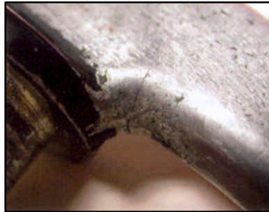
Cracked and broken steering arm (Bruce White)
